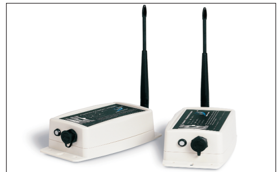
AeroComm's ACE RF modems are housed in a rugged NEMA-4x enclosure.
